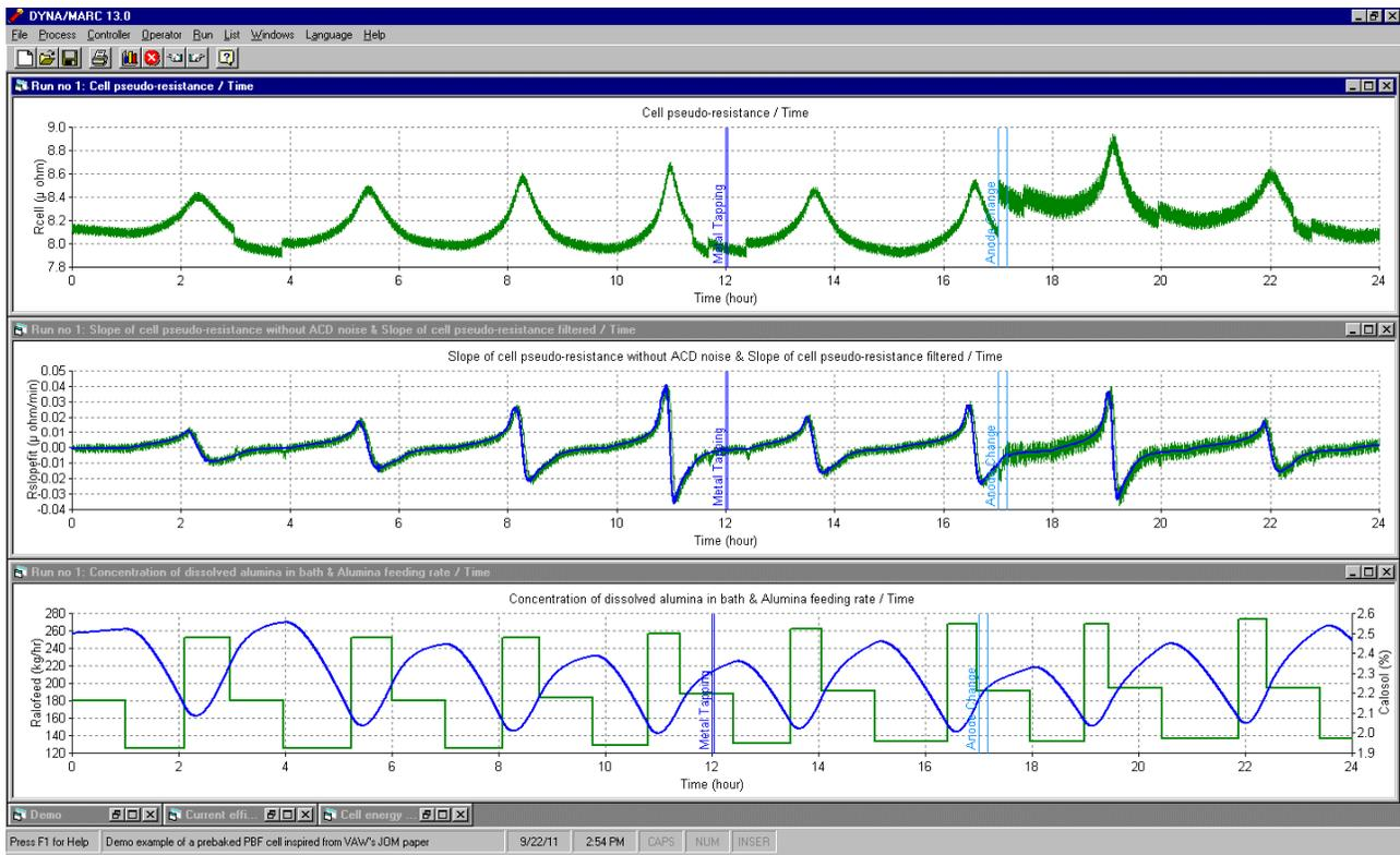
Figure 7: 24 hours Dyna/Marc simulation using the Demand Tracking Feed Control
