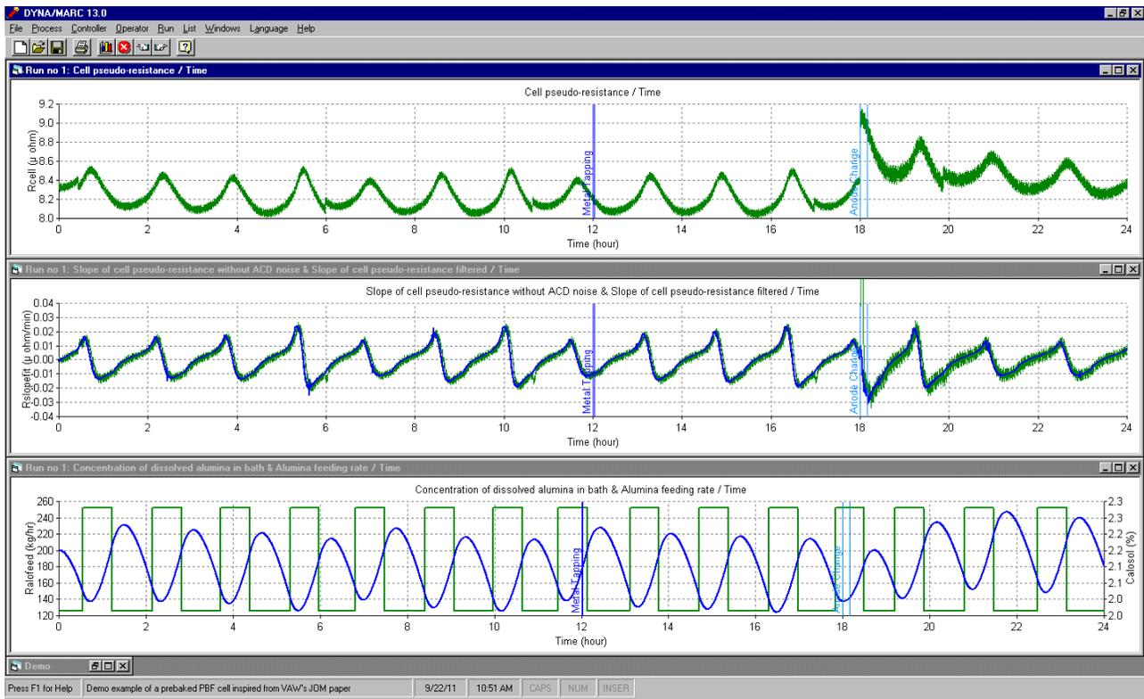
Figure 5: 24 hours Dyna/Marc simulation using the Pechiney Tracking Feed Control, shorter cycles
