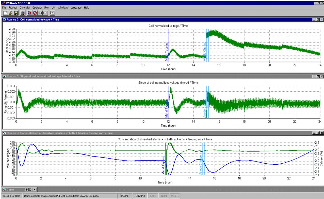
Figure 13: 24 hours Dyna/Marc simulation using the *In Situ* Feed Control with normal anode change event
