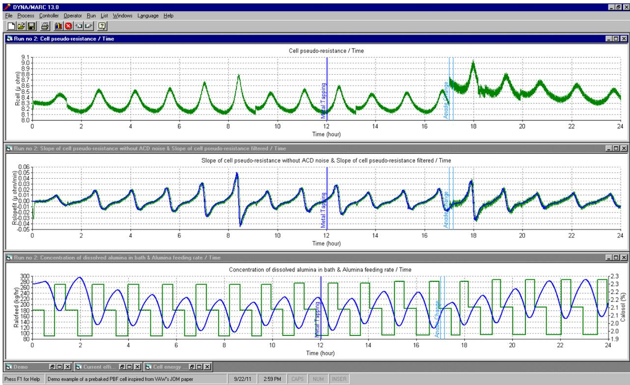
Figure 9: 24 hours Dyna/Marc simulation using the Demand Tracking Feed Control, shorter cycles
