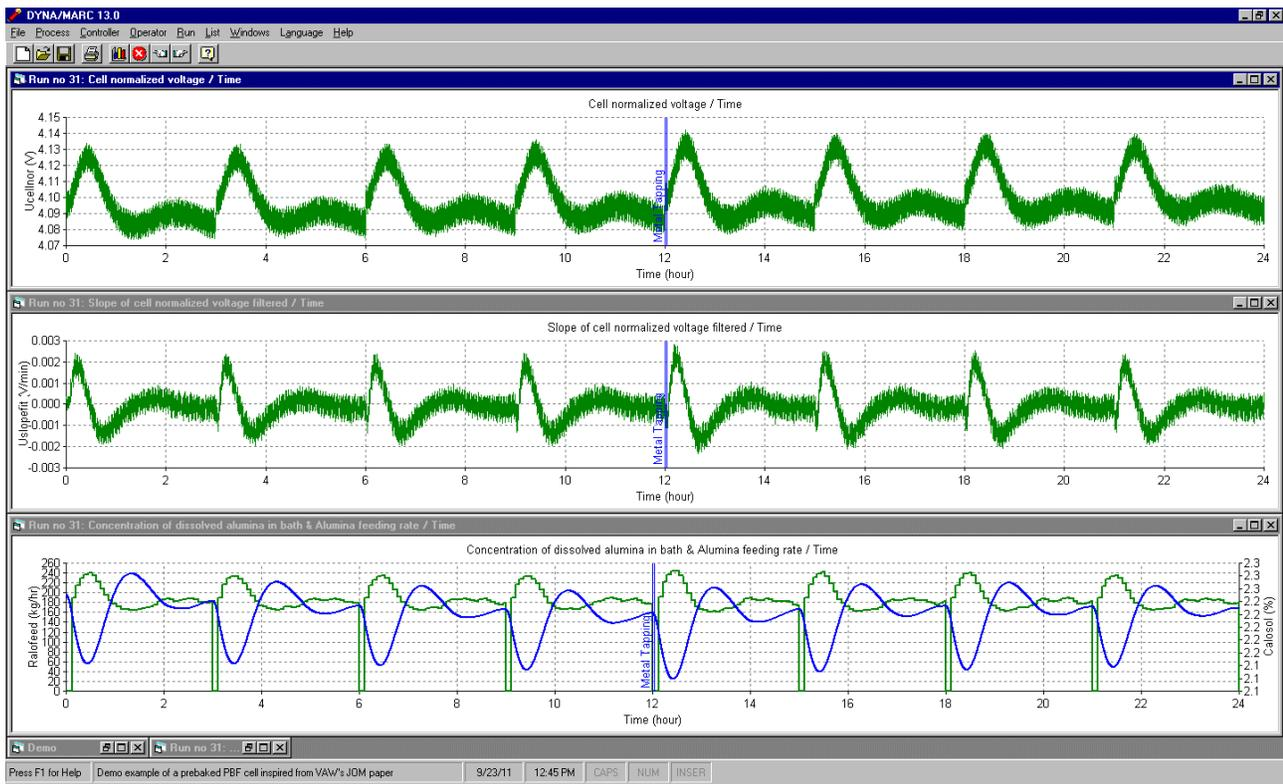
Figure 11: 24 hours Dyna/Marc simulation using the *In Situ* Feed Control
