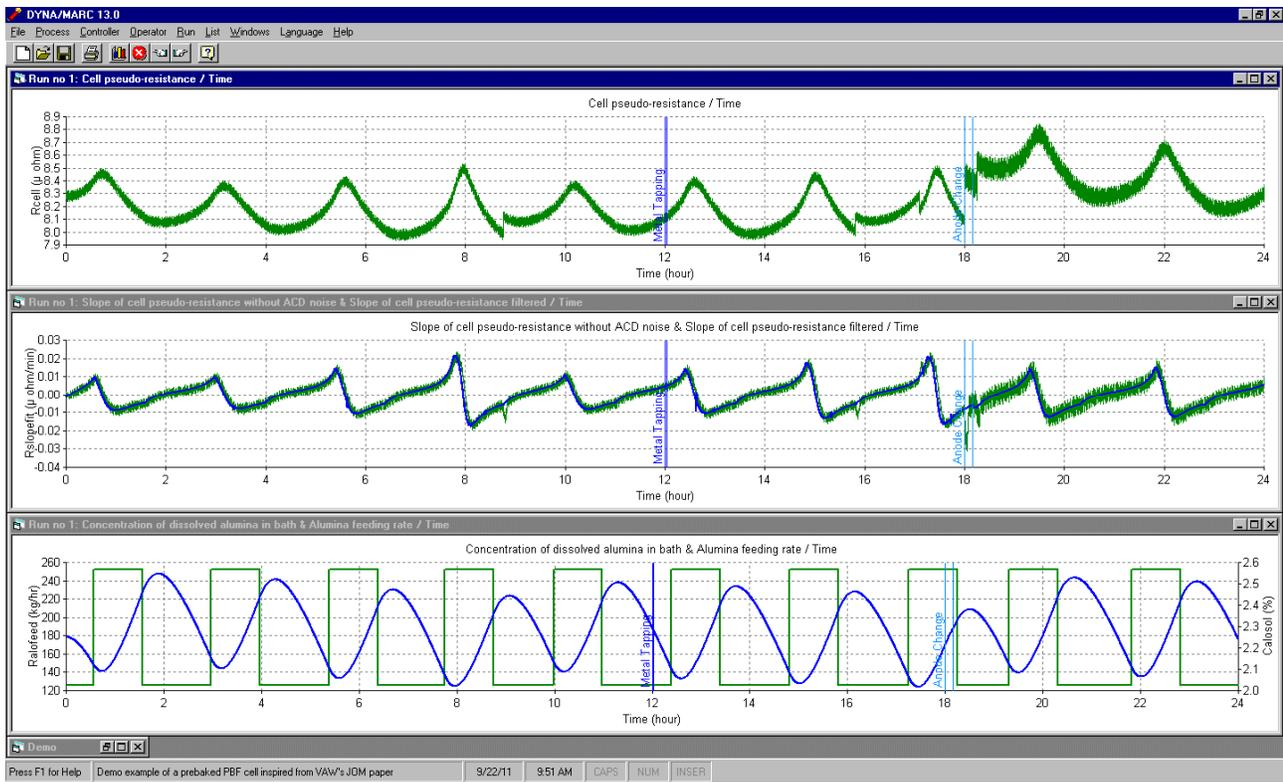
Figure 3: 24 hours Dyna/Marc simulation using the Pechiney Tracking Feed Control
