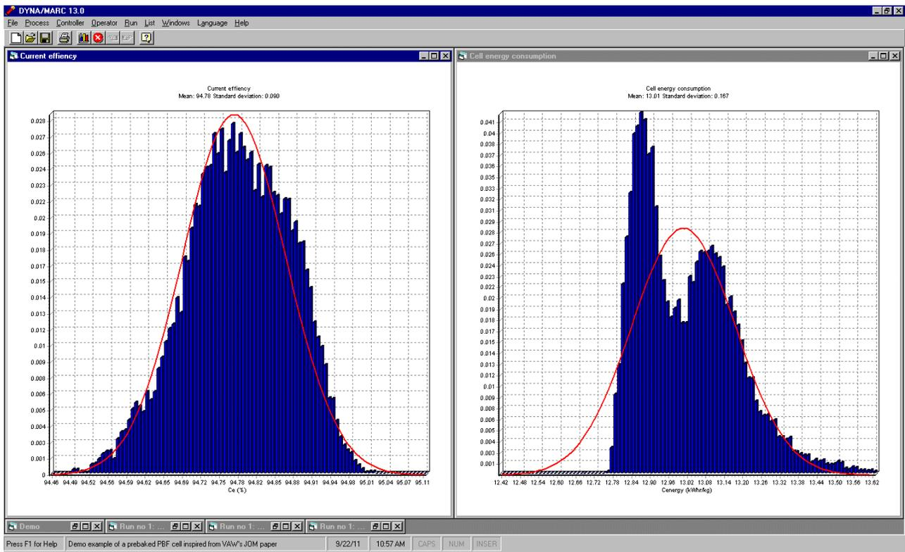
Figure 6: Predicted 24 hours averaged cell power and current efficiency, using the Pechiney Tracking Feed Control, shorter cycles
