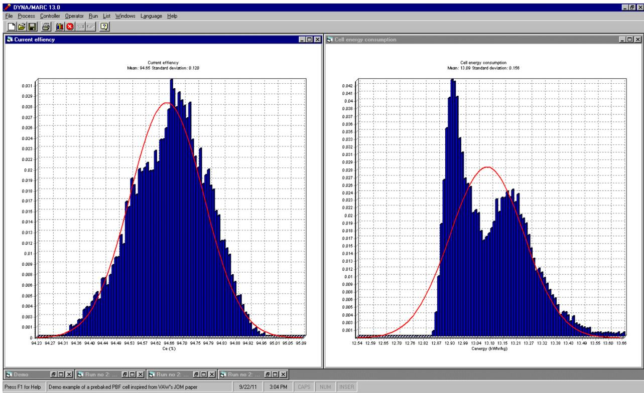
Figure 10: Predicted 24 hours averaged cell power and current efficiency, using the Demand Tracking Feed Control, shorter cycles
